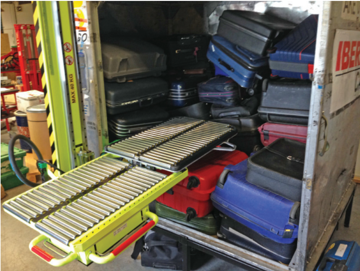
The picture above shows the CUS. As you can see it is slightly leaning to maximize the emptying speed.
